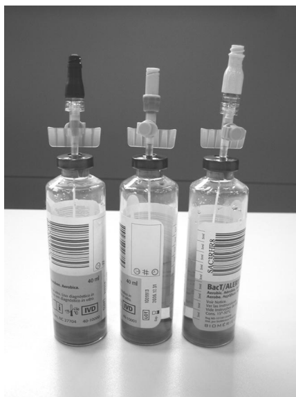
Figure 2. The experimental model consisted of a bottle of aerobic blood culture (Bact/alert, Bionerieux Inc, Durham, NC) into which an 18G peripheral venous catheter (Venflon) was inserted. We used disinfectable needle-free closed connectors from three different manufacturers to close the catheters.
